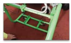
There are two clips on the bottom base to hold the air compressor. The typical gun uses an air gun so that is why you would need the air compressor.
