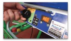
Typically you're going to run between 3-5. The higher you turn it up the higher the pressure is. The lower you turn it the lower the pressure.
