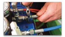
Be sure to carefully tighten each hose connection.
