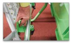
Make sure the clips are down and in place so that when you tilt your cart up the pump does not fall out. There are 2 clips are in the back and one in the front center below with pressure gauges.
