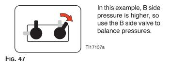
**NOTE:** Turn Recirc/Spray valve only enough to balance pressure. If turned completely, all pressure will bleed off.
