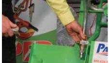
Make sure to note that this male plug goes into the female insert in the barrel for the B-Side barrel.
