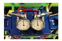
Both gauges are at the 12:00 position for spraying.
