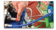
The Pressure line is where the red caps on the back where the hoses get connected. (The B-Side is shown here.)
