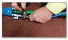
Make sure to tighten each connection lightly.
